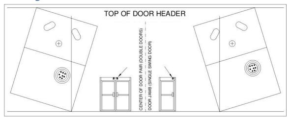
Mounting of your Surround Sensors involves mounting the supplied bracket to the door frame above the door handle, angling it towards the lower adjacent corner. On double swing doors the same this installation is repeated for both sides. For accurate mounting angle use our bracket mounting template.
