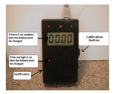
On the left side of the calibrator, slide the power switch up (on). The first two digits on the LCD display indicate the red channel, the second two digits indicate the green channel. Activity on either of these channels is indicated by the corresponding LED above the display.
