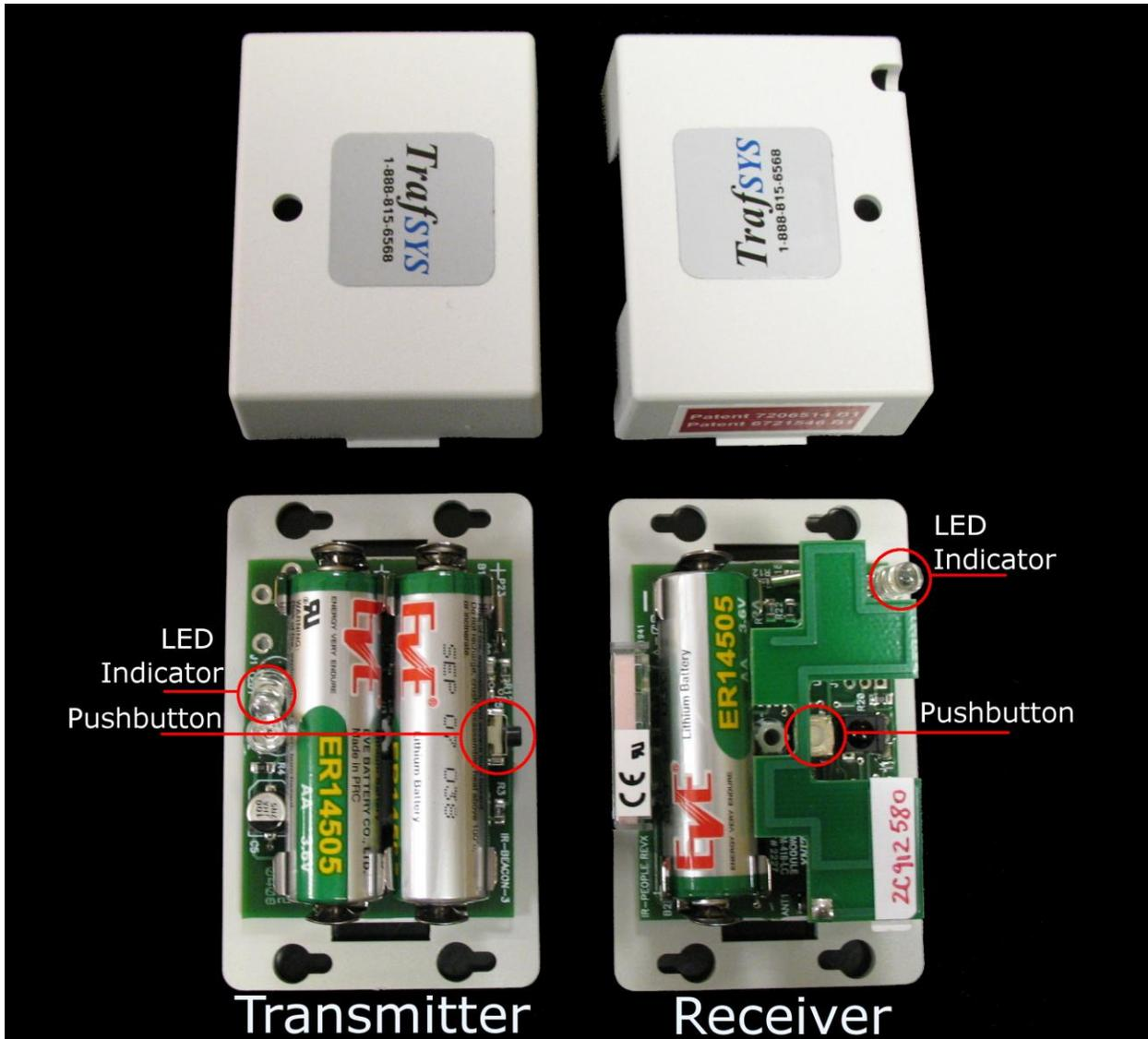
Figure 3: TrafSYS Front Firing Wireless Beams
