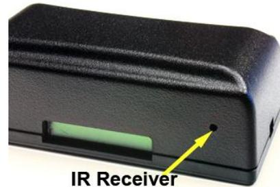
To put the counter into Alignment Mode, momentarily press and release the configuration button on the IR Receiver. If the IR Receiver and IR Transmitter are properly aligned, then the LED will be lit on the IR Receiver. You can exit Alignment Mode by pressing the Configuration Button again or allow it to exit Alignment Mode on its own (after 60 seconds). This button is also used to send a service packet. This will be discussed later in the manual.
