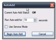
The "Use Service Mode" option will add only sensors that are sending a service packet.
