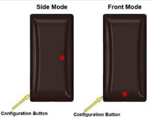
To select the mode of operation, use a paperclip to press and hold the configuration button. The visible LED's will provide feedback to the available modes (Side Low Power, Side High Power, Front Low Power, Front High Power. Low Power Mode is indicated by a solid LED and High Power Mode is indicated by a flashing LED.
