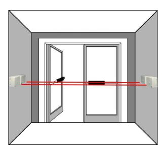
Figure 1: Typical Directional Beam Installation
