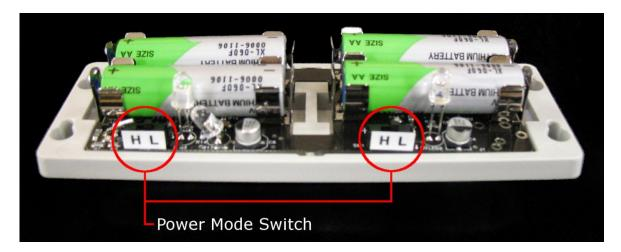
Figure 4: Power Mode Switch
