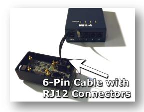
The 8 LEDs that appear on the front of the MIU-4 indicate activity on each of the ports. You will see each LED flash for the corresponding port when data is being sent to the MIU-4. If the LED should appear solid, this indicates that there is a short in the wiring to this port and you should check your pairs to make sure the wiring is straight-through end-to-end.
