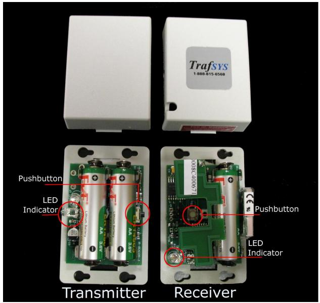
**Figure 4: Trafsys Side Firing Wireless Beams**
